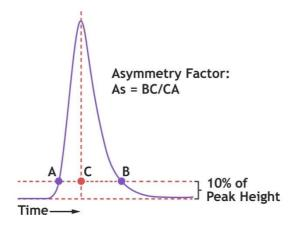
7. The recommended asymmetry factor for packed anion exchange adsorbents is between 0.8 to 1.2. The recommended plate count for an acceptable pack is  $\geq$  2000 N/m.
